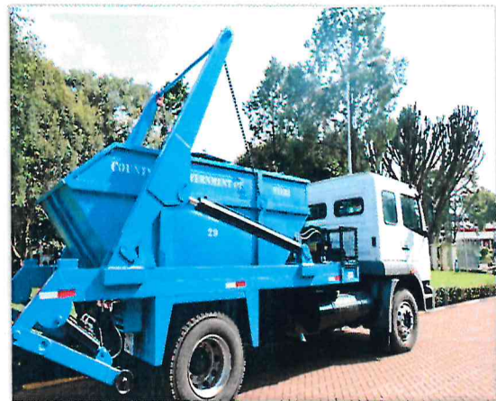
Fig 2: Skip loader waste truck
